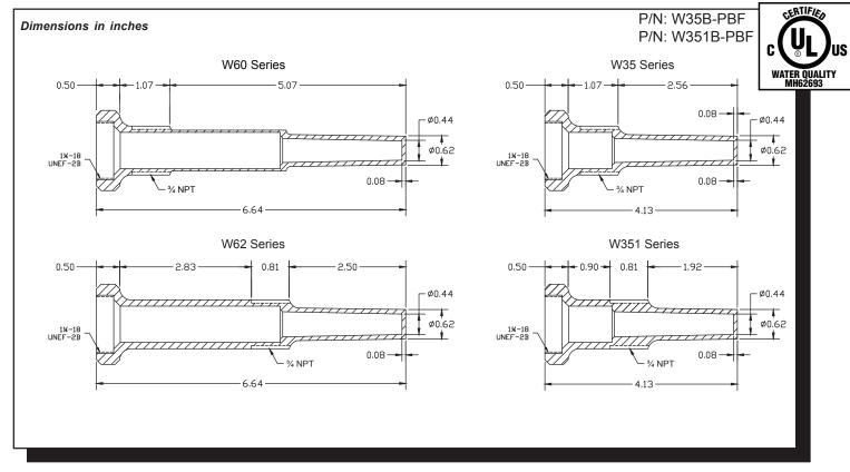
These thermowells are designed for use with Miljoco liquid-in-glass and solar industrial thermometers. They are intended to separate and protect the thermometer from the process or media being measured and allow for the removal of the thermometer without shutting down the process. They are readily available in brass, lead-free brass, type 304 stainless steel, or type 316 stainless steel construction to suit a wide range of applications. Other materials are available on request - consult factory.
