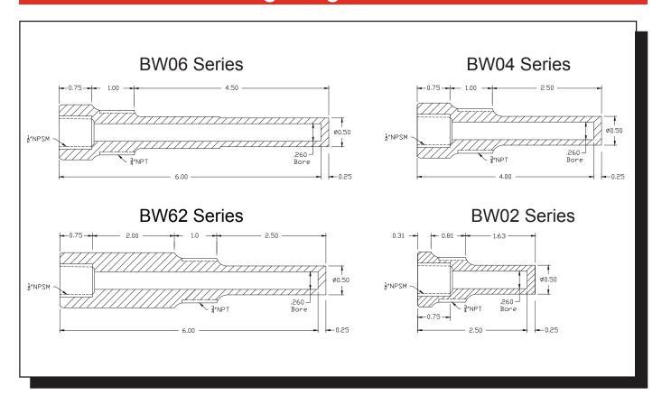
These thermowells are designed for use with Miljoco 3" & 5" Bimetal Thermometers. They are intended to separate the thermometer from the process or media being measured to allow for removal of the thermometer and protection of the thermometer stem from corrosive media. They are readily available in brass, 304 stainless, or 316 stainless steel construction to suit a wide range of applications. Other materials and designs are available on request - consult factory.
