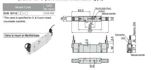
2-Position, 3-Port, Double Solenoid Valve Connector Lead-Out Direction: Side (Valve for 5-port mixed mountable type)
