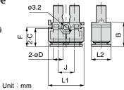
1/8 14.1 22 12 11 10 11.1 PQ1/8M-A 3.8 PQ1\_8M-A 14.1 22 12 10 PQ5/32M-A 5/32 11 11.1 3.6 PQ5\_32M-A PQ1\_4-A PQ1/4-A 1/4 17 22.4 29 17 14 18.9 21 5/16 PQ5/16-A 20.7 29 17 18.1 14 17.2 PQ5\_16-A 14 PQ3M-A 3 14.1 22 12 11 10 11.1 PQ3M-A 3.8 PQ4M-A PQ4M-A 14.1 22 12 11 10 11.1 3.6 4 PQ6M-A PQ6M-A 14.5 22 12 11.6 10 11.5 6 4.3 20.8 29 17 17 14 17.3 13 PQ6-A 6 PQ6-A PQ8-A 8 20.7 29 17 18.1 14 17.2 14 PQ8-A
