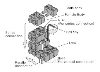
\* Standard type can not be connected with mini type
