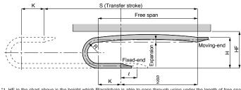
\*1. HF in the chart above is the height which Plarailchain is able to pass through using under the length of free span with allowable expansion without load such as cables, hoses, etc \*2. Please make inquiries for special travel conditions.
