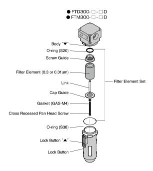
(2) For Filter Element Set "FE300D (for 0.3µm)" or "FE300M (for 0.01µm)"
