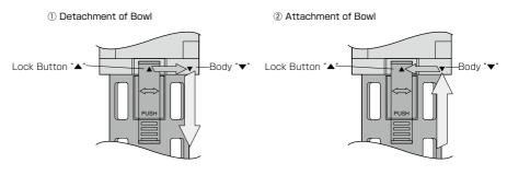
5-2. Filter Replacement (Refer to figures) 1)5µm Element (FTA300-□-□D)
