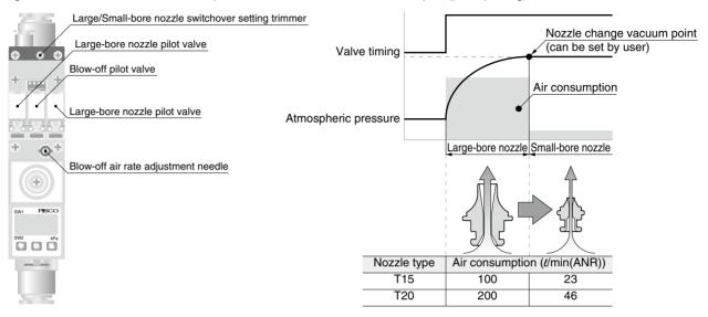
• The two-stage nozzle type's vacuum suction rate has been increased by approximately 40% compared to conventional types (PISCO Vacuum Generator complex type with single nozzle).
