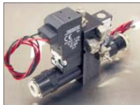
This distinctive valve assembly features a pressure regulator, two solenoid valves, a needle valve and fittings with precision orifices
